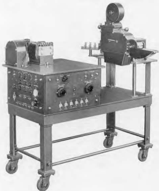
A three-element camera oscillograph with the self-developing feature
