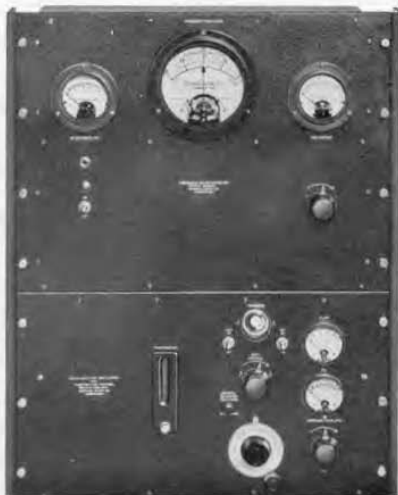
FIGURE 1. The frequency monitor consisting of a TYPE 575-D Piezo-Electric Oscillator and a TYPE 581-A Frequency Deviation Meter
